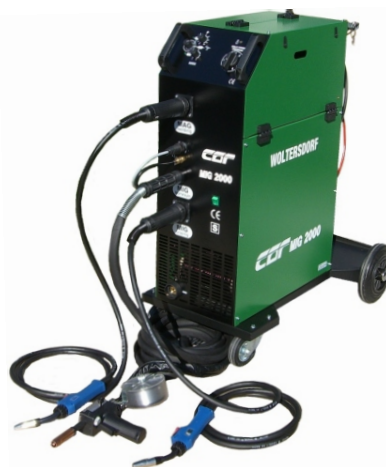
CARMIG 2000: 3 welding torches for MAG welding, MIG aluminium, MIG brazing
